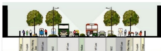
Figure 7 Ideal NMT incorporated road section. [12]
